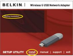
**Note:** If the Belkin Wireless Networking Utility screen does not appear within 20 seconds, access your CD-ROM by double-clicking on the "My Computer" icon; then, double-click on the CD-ROM drive into which the installation CD has been placed. Double-click on the folder named "Files", then double-click on the icon named "setup.exe".
